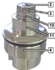
Fork cap with reversed preload
