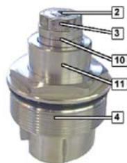
Fork cap with reversed preload
