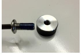
2) Insert the provided bolt in the hole at the upper rearmost side of the brake pedal.
