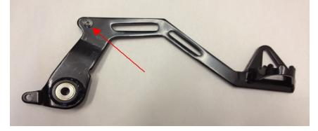
3) Thread the provided spacer onto the bolt at the back side of the brake pedal.
