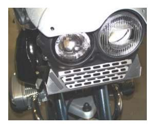
Loosen the two outside screws, which serve as the mounting of the headlight screen.
