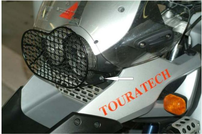
Installation: Remove the original attachment screws of the black plastic headlight side bezel.
