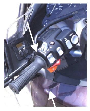
The handlebar mount can employ any of our mounting plates. The model used for example is the K1200LTbut will work also with the R1100RT and R1150RT.
