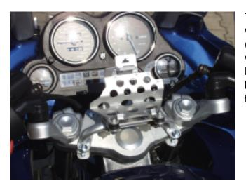
The mount adapter for the BMW K1200RS is put on with the handle to the rear on the fork bridge. (in driving direction) The screw connection takes place with the two enclosed shims, the four cap head screws M5x45 with small M5 washers above, large M5 washers below as well as the four self-locking M5 nuts under the fork bridge.
