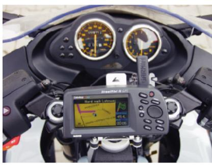
Put the mount adapter on the upper fork bridge, with the longer attachment tabs to the rear. Pass the two plates under the upper fork bridge one at a time, and hold while passing the bolts through the mount adapter tab and the plate. Use a washer and M6 locking nut on each bolt. The adapter is above the fork bridge, the two plates are below the fork bridge.
