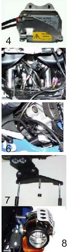
Assembly of the controller: Locate the controller with the padded side downward and with the cable exiting left from the bracket.(Photo 4) Fasten the mounting plate for the solenoid with two bolts M5x45 LiKo and two spacer rolls of 10,5,37
