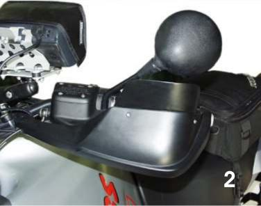
Attach the spoilers with supplied M4x12 dome head screws, washers and nylock nuts on the hand guards.
