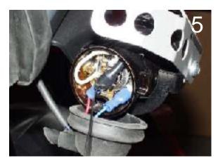
Shorten the blue and red cable to correct lengths and pull them through the two paths planned for them to the lower part of the foglight rear cover. Attach the provided flat pins to the cables. Plug the blue cable into the foglight on the outside right. This is the ground wire.
