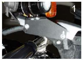
First you must bolt the fog headlight unit to the provided bracket with two caphead M6x12 screws and washers. Now screw the light and bracket onto the front support at the right on the original fender attachments with two caphead M5x20 screws and washers. Put two small M5 washers between bracket and fender. Screw connections together loosely, the headlight adjustment is done with these later.(Photo 1)
