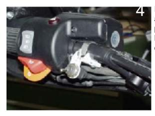
Electrical connection: Bring the switch to the handlebar and install it at the left side directly beside the clutch perch with the provided clamp, two caphead screws M4x10 and two nuts M4. Adjust the switch so that it can be flipped vertically. (Photo 4)
