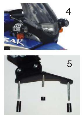
Pull the red and blue cables to the right side of the upper covering. Install tank cover, side panels and headlight again. Bolt the fog headlight to the mounting plate with the two LiKo M6x14 bolts and washers. Bolt the fog headlight bracket to the right blinker mount with 2x LiKo M5x45, 1x LiKo M5x25 and the spacer rolls (24 in the back, 07 center, 19 in front). Bolt in the original screen screw connections (fig. 5). Reattach screen with the LiKo M6x10 and washers.
