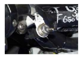
Bring the switch to the handlebar and install it at the left side directly beside the existing switch with the provided clamp, two screws LiKo M4x10 and two nuts M4. Adjust the switch position so that it can be flipped vertically. (Photo 3) Bring the brown cable to negative pole of the battery. Shorten to suitable length and attach the cable to the round adapter eye. Do not connect yet.
