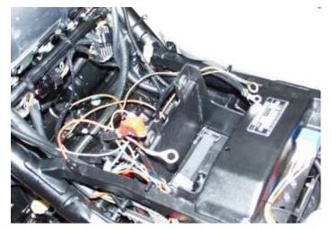
Route the green cable to the battery negative (ground) pole.
