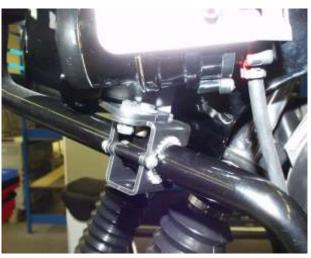
Route the switch to handlebar and attach it on the left side next to switch gear with supplied clamp, two dome head screws M4x10 and nylock nuts M4. Adjust switch so that it can be operated vertically.
