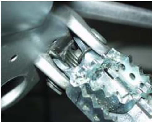
**Installation:** Remove the split pin on the under side of the foot peg holding bolt and pull then the bolt out.
