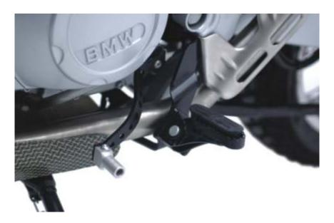
Loosen the clamp screw on the original shift lever and remove it from the lever. Now you can remove the stock shif lever. It may be difficult to pull out so you can carefully pry the clamp gap open with flat head screw driver.
