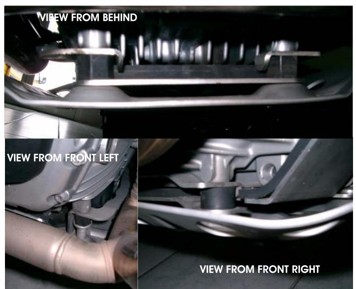
Remove the BMW original motor guard and the rubber isolated bolts/spacers. Put the reinforcements on the motor and reattach them with the orig. rubber isolated bolts so that the longer side of the rubber isolated bolt thread point downwards.
