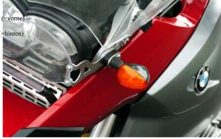
Lay the Touratech blinkers in each corner of the bike so that the small hole between the blinker glass and black housing is facing down (drainage/opening hole).
