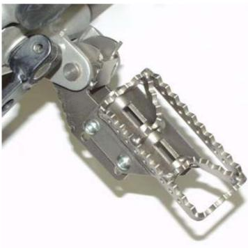
Tighten the six M6 buttonhead screws to 10 Nm. Check tightness after 30 miles. For all other connections please refer to manufacturer recommendations.
