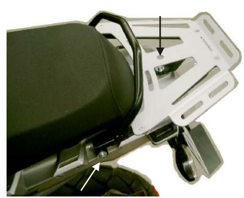
Note that weight on the rack may change the handling characteristics of your motorcycle. Maximum weight on the rack is 5kg or approx. 10lbs
