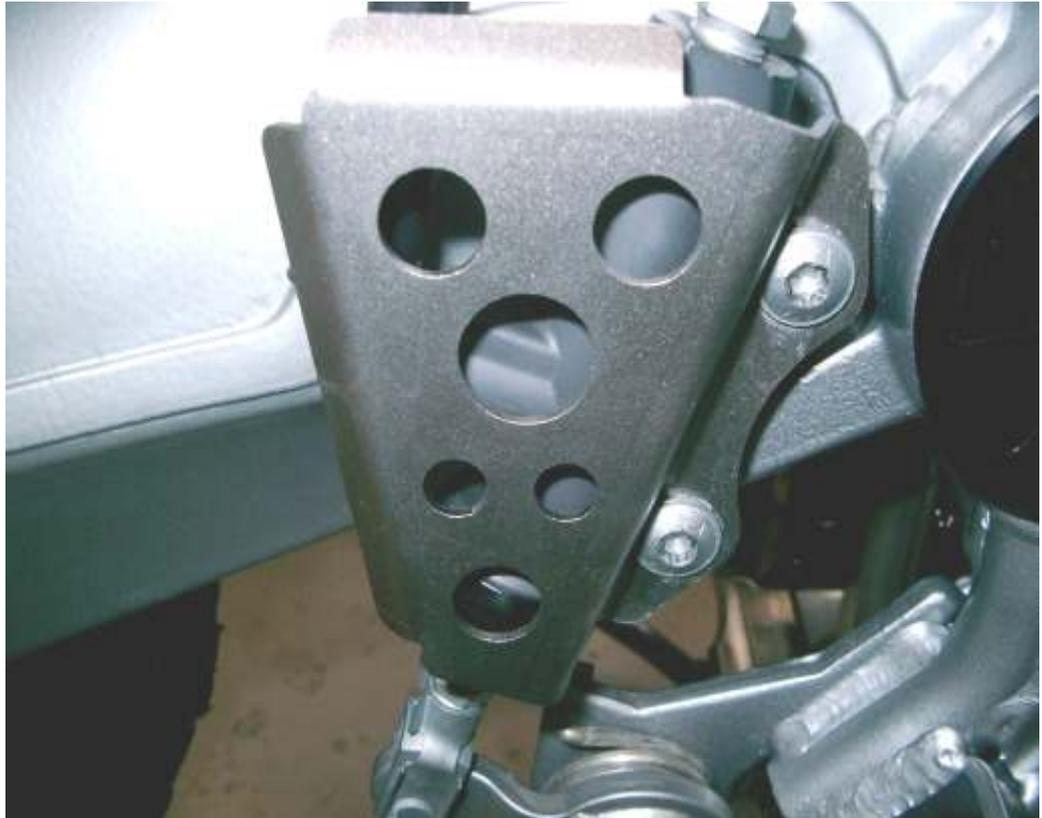
Remove the original BMW guard and install the Touratech stainless steel guard with original hardware.
