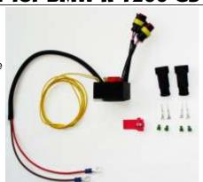
Route the yellow cable to the tail of the motorcycle. Remove the cover of the tail lightand route the yellow cable thru the rubber grommet into the tail light and connect it there with cable connectors to the tail light (pay attention to the markings on the wires). Make sure to attach it to the tail light wire and NOT the brake light wire.
