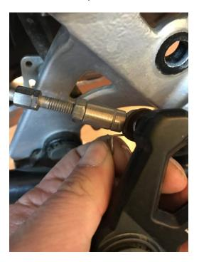
**Step Three:** With the clip removed hold the shift linkage, and roll the lever until it pops out of the shift linkage.
