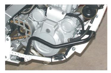
Photos above show F650GS with TOURATECH kits: Raised Engine Underbars 300-0042 and Footrest Relocation Kit 300-0041.
