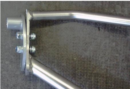
2) Remove the Torx T-30 screw on the left side of the bike that holds the oil line. On some bikes you may need to loosen lower screw as well if the crash bar mounting hole does not align quite right. The crash bar will be attached here with M6x20 and washers M6 on both sides. Make sure that the attachment is correctly aligned in the frame.
