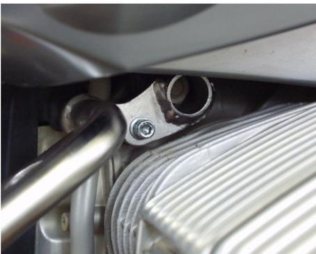
Torque the bolts finally to BMW specs at 9Nm.
