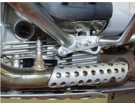
Torque the bolts finally to BMW specs at 25Nm.
