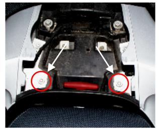
Exchange the two marked screws on the inside of the luggage compartment for the two enclosed allen screws M6x35 with one large M6 washer each. You must fully tighten these two screws before further mounting, since the screws fit in threaded mounts in the subframe and cannot be pulled tight later.
