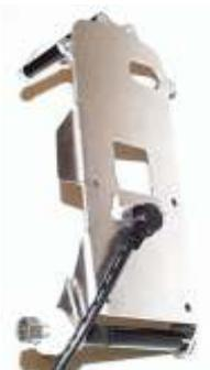
Touratech GPS mount is vibration isolated with rubber spacers. Make sure no other part of the GPS or the GPS mount is touching the handlebar or other parts on the bike for best protection against vibration damage.
