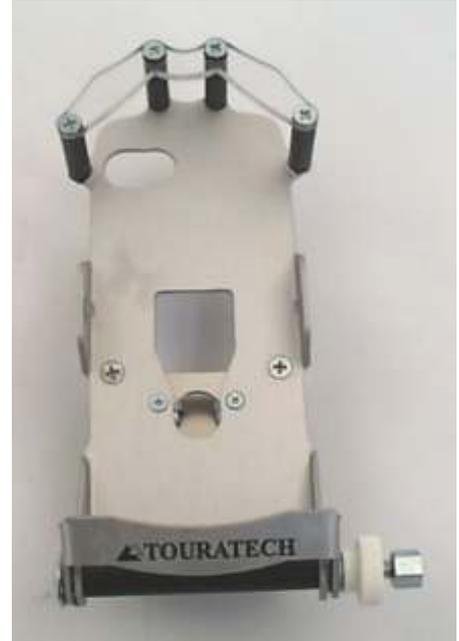
Open the GPS mount by untightening the white plastic thumb nut. Now turn the latch with Touratech text up and open. Set the top of the GPS unit in the mount and then the bottom down. Turn the latch closed against the GPS unit and retighten the white thumb nut. Check that the latch is tightly closed and the white thumb nut tightened in regular intervals during the ride !
