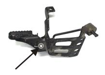
Remove the split pin and washer from original footrest pivot. Note the configuration of the footrest return spring.
