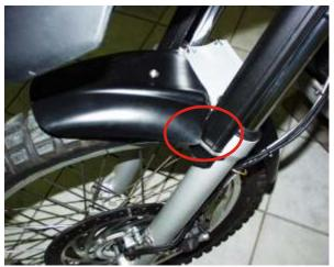
Note: Low fender needs to be cut so that the fork protectors can move free (3rd photo)
