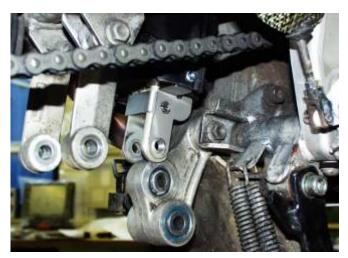
Reattach the bottom linkage point with the supplied M12 nylock nut to BMW torque specs. Do not forget to check that the bearing dust covers are properly in place.
