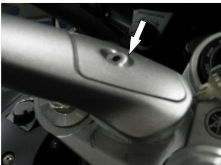
16. Now reattach the original coverings of the handlebar fastening bolts using the respective M4 bolts.
