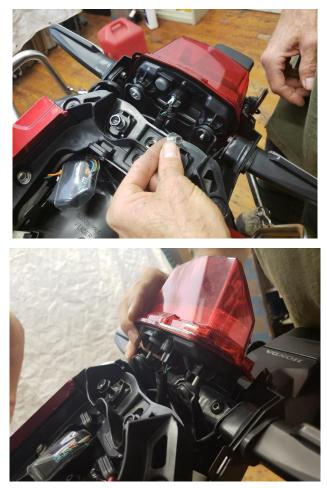
• Disconnect the tail light wiring (orange and blue plugs).
