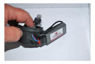
• Plug in your headlight into the motorcycles wire harness and carefully work the connector into the headlight housing.
