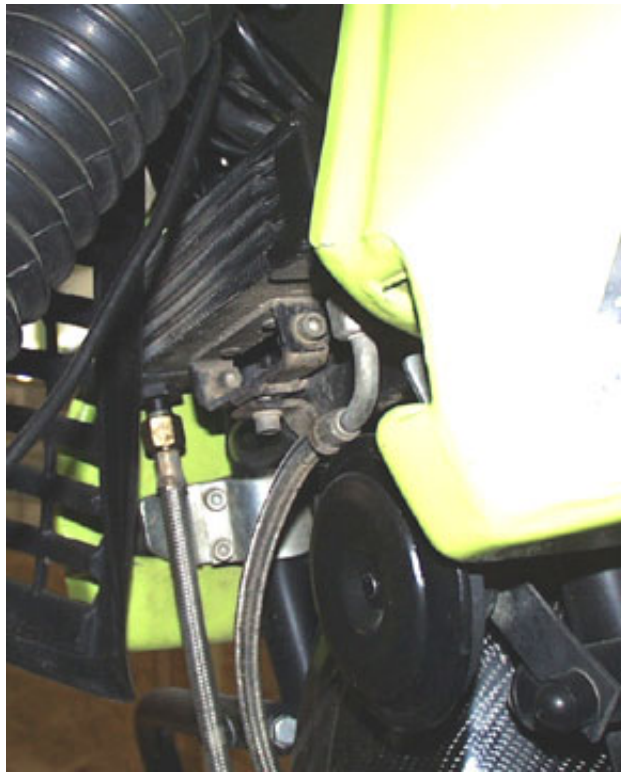
Diagram 2: Showing center position of oil cooler. A ventilated fender is available ( 040-0220 black or 040-0221 white).
