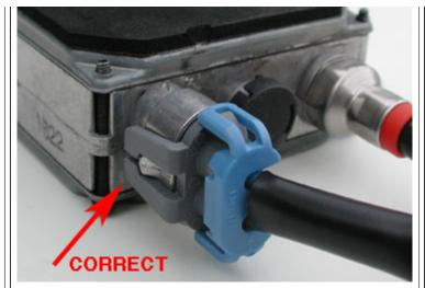
**Correct connection** of power supply to the ballast. Gray fingers easily slide past and engage on wedge-shaped protrusion.
