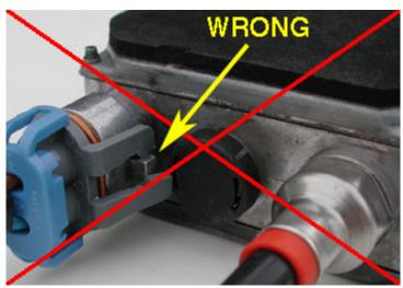
**WRONG connection.** Forcing the gray fingers over the square barrier and then applying power will cause a non-warranty failure of the ballast.
