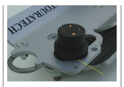
Press the cord into the cutout. It fits exactly, very German and very perfect. NOTE it is NOT possible to install the GPS into the mount then insert the power cord.
