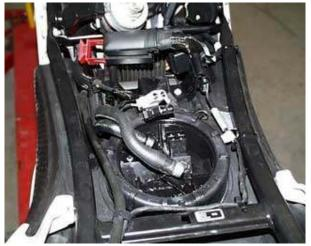
1 3 CAREFULLY disconnect the fuel lines. There may still be pressure in the fuel lines that will cause them to leak some fuel. Plug the fuel lines to prevent any contamination from getting into them.
