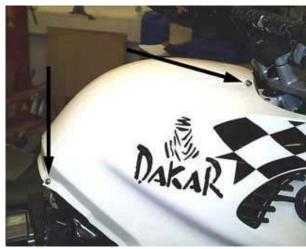
Remove the two screws that secure the top of the cover. (Torx 25)
