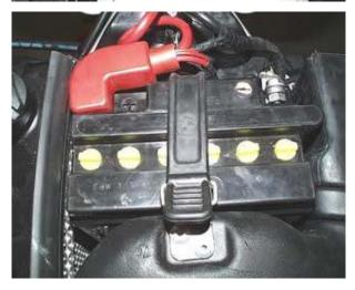
Remove the battery cables from the battery using either 2) 10mm open end wrenches, or a wrench and a Phillips screwdriver. Remove the battery vent hose, disconnect the strap and lift the battery from the tray. Always keep the battery level. NOTE: Battery acid is corrosive and is hazardous to your health!!
