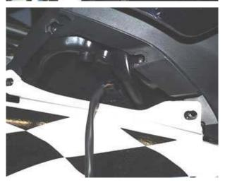
Squeeze the sides of the connector to release it and pull to disconnect. Do not damage the wires from the turn signal, we will be reusing these. Follow the same steps to remove the other turn signal.
