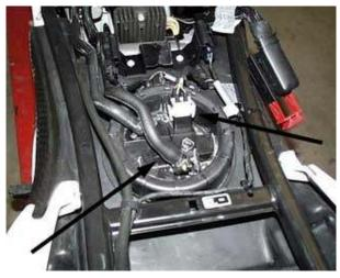
Remove the two electrical connectors from the fuel pump. Loosen the screw type clamp on the fuel line. Cut the band clamp from the second fuel line. A new screw-type clamp is included to replace the clamp that was cut.
