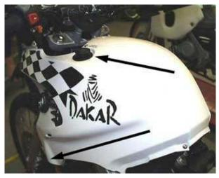
On the left side, remove the oil cap. Pull outward on the lower forward edge of the cover.
