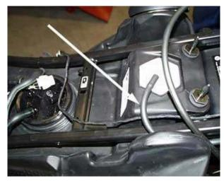
Because the new forward tanks are much higher, the charcoal cannister must connected to the new forward tanks. (see photo on step 30)
