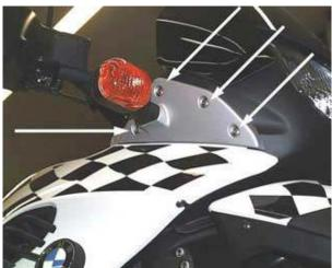
Remove the front turn signals. Remove the 4 (Torx 25) screws securing the turn signals to the faring. Pull the light assembly away to expose the electrical connector.
