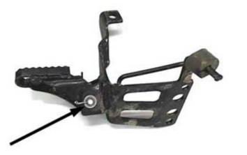
Remove the original foot pegs from the mounts. Remove the cotter pin and washer then push the pin out of the mount. The pins, spacers, springs, and washers are reused. Disassemble both the right and left foot pegs.
