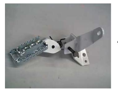
The new foot pegs are now installed into the new foot peg mounts using the original hardware we just removed. Place the spacer and spring in the center of the foot peg, now place the peg into the mount with the bent end of the spring into the hole in the mount. Hold the foot peg in place and install the pin. Place the washer on the bottom and install a new cotter pin.
