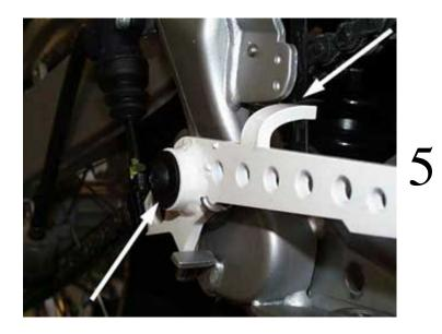
positioned above the brake pedal. The bolt can now be tightened to 15ft/lbs. Reconnect the rod from the master cylinder using the original clip. The shifter can now be installed on the left side. (5mm Allen key)
