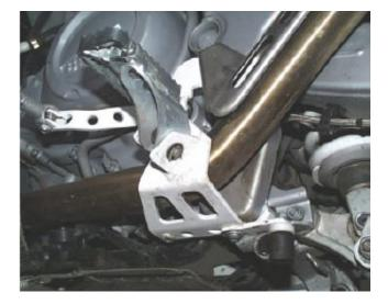
On the right, install the new foot peg mount with three original M8x20 button head bolts (Torx T40) and the original washers.
