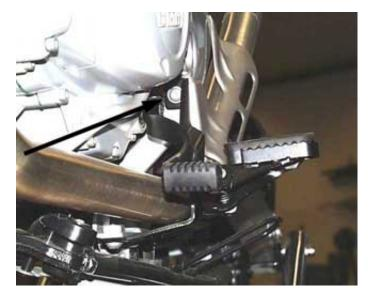
Remove the foot peg mounts. There are three bolts (Torx T40) holding each foot peg bracket to the frame. Remove the three bolts and the bracket along with the foot pegs.
