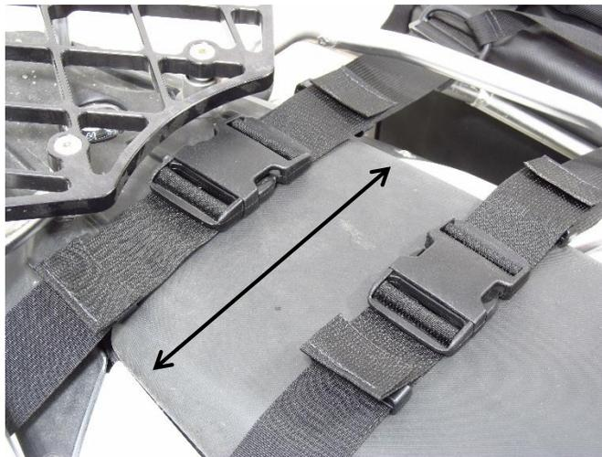
**Always use the seat straps.** The Rocky Mountain Saddle Bags and racks are designed for these, as the seat straps distribute the weight of the bag. Failure to use the seat straps can result in damage to the bags, motorcycle and bodily harm. This will also void any and all warranties.
