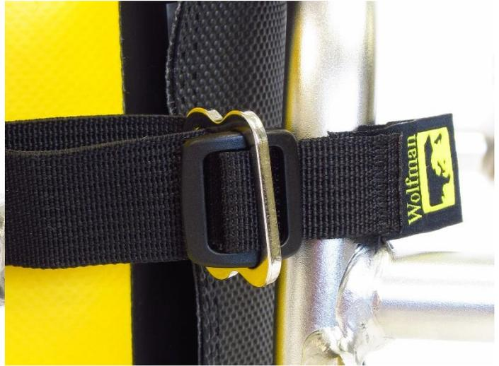
5- Tighten the 1" Mounting strap which will tighten the saddle bag strap and the 3/4" slide is captured, as shown in FIG.8
