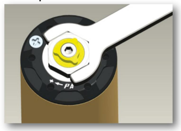
The spring preload is fundamental for the function of the suspension. If the preload is incorrectly set, any other adjustments will not help to get the intended performance from the
